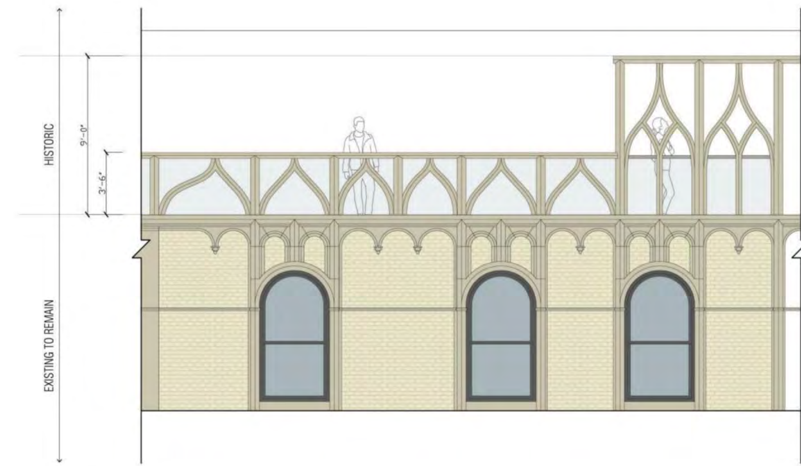
E1 HISTORIC PARAPET ELEVATION SCALE: 3/16"=1'-0"
