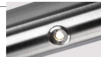
X2: CONTINUOUS S.S. HANDRAIL WITH INTEGRATED 3.5' O.C. 3000K IP67 LOW PROFILE LED LUMINAIRE
