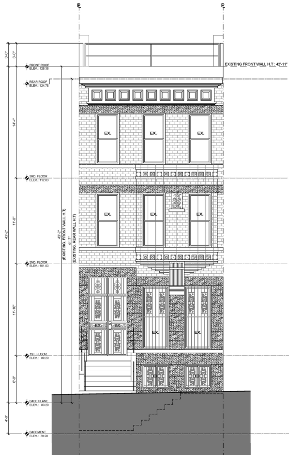
FRONT ELEVATION BEFORE WORK
