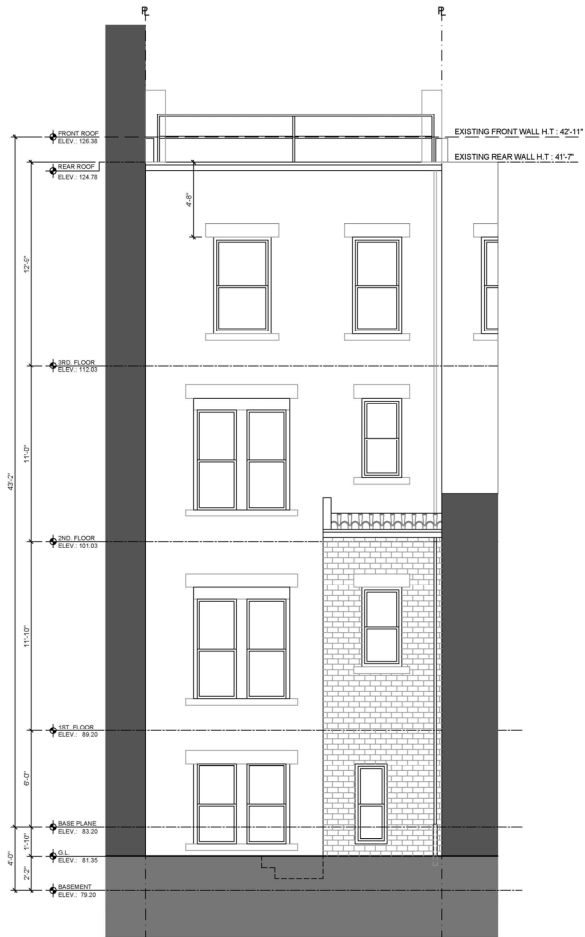
REAR ELEVATION BEFORE WORK
